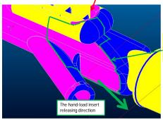
A. We may revise the draft for the hand-load insert releasing. The area of the hand-load insert is in the green curves.
