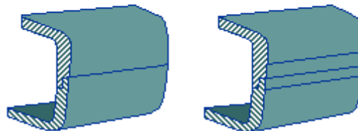
Matching Tongue and Groove Align Two Parts
