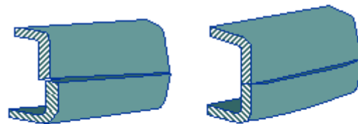
Butt Joints Are Difficult To Align
